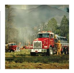
Vehicles used in firefighting applications are often exposed to airborne burning embers. If these burning embers are drawn into the engine air intake of a piece of equipment, they can burn holes or ignite the paper in the air cleaner filter. This event can cause severe engine damage, leaving the vehicle or equipment inoperable.
